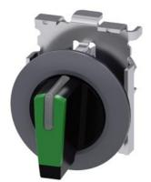
Selector switch, illuminable, 30 mm, round, Metal, matte, green, selector switch, short, front ring for flush installation, 3 switch positions I-O-II, latching, actuating angle 2x45°, 10:30h/12h/13:30h, with laser labeling, inscription or symbol Customer-specific selection with SIRIUS ACT configurator (CIN)
