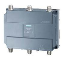
IWLAN Access Point, SCALANCE W788-2 M12, 2 radios, 6 N-CON antenna port, iFeatures support via KEY-PLUG, IEEE 802.11a/b/g/h/n, 2.4/5GHz, gross 450 Mbit/s per radio, 1x M12 max. 1 Gbit/s, PoE, redundant 24 V DC,M12 A-coded IP65, -20..+60 °C, plug slot, WPA2/802.11i/e, observe national approvals! CERT ID: RAPN-W2-M12-E3, includes: MPCIE-R1-ABGN-U3, scope of delivery: Manuals on CD-ROM, German/English, M12 sealing caps, only for operation in the USA.
