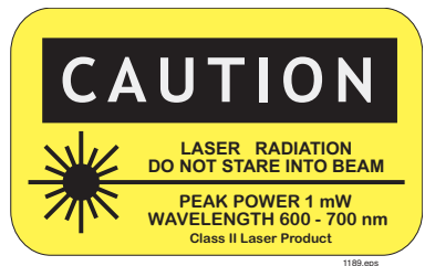
Figure 4. Warning logotype label for Class II lasers.
