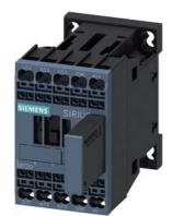
power contactor, AC-3 12 A, 5.5 kW / 400 V 1 NC, 24 V DC 0.7-1.25\* US, with varistor plugged on, 3-pole size S00, spring-type terminal not expandable with auxiliary switch
