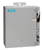
Pump control panel, Size 1, Three phase full voltage, Solid-state overload relay, OLR amp range 10-40A, 208VAC 60Hz coil, Standard type contactor, 30A circuit breaker, HOA Sel Sw. <(>&<)> Start P.B., Enclosure NEMA type 3/3R, Weather proof outdoor use
