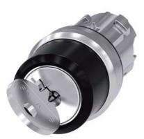
RONIS key-operated switch, 22 mm, round, metal, shiny, lock number SB30, with 2 keys, 2 switch positions O-I, latching, actuating angle 90°, 10:30h/13:30h, key removal O+I, possible special locks: SB31, 421, 455, with laser labeling, lower case
