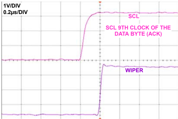
FIGURE 21. WIPER LARGE SIGNAL SETTLING TIME
