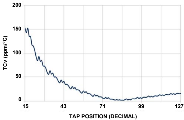
FIGURE 13. 10kΩ TCv vs TAP POSITION, V_{CC} = 3.3V
