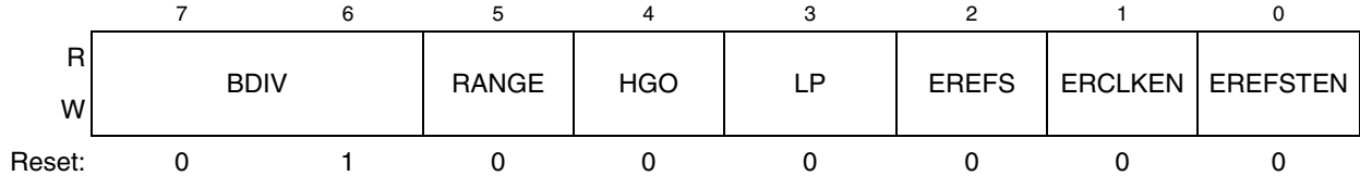
Figure 10-4. ICS Control Register 2 (ICSC2)
