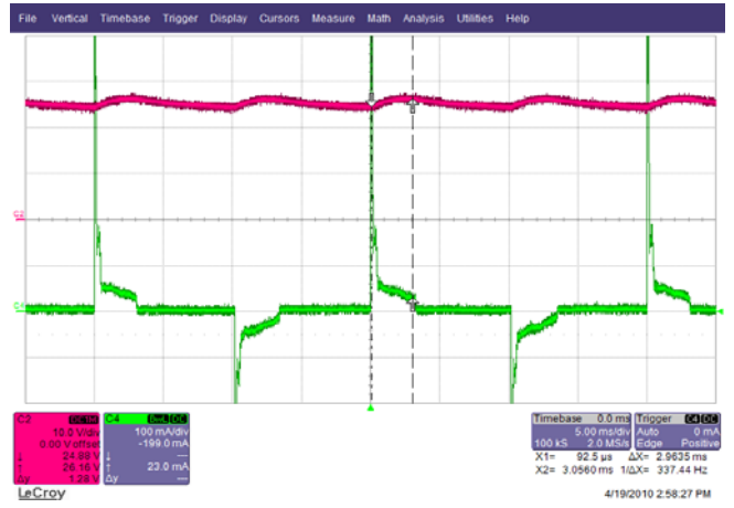
Figure 35 – 230 VAC, 54° Phase. Upper: V_{OUT} , 10 V / div. Lower: I_{IN} , 0.1 A / div., 5 ms / div.
