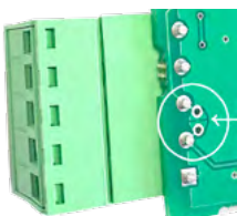
On the back side of PCB, cut track of pin 1 and pin 2 for differential function
