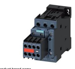
Power contactor, AC-3 32 A, 15 kW / 400 V 2 NO + 2 NC, 24 V DC with plugged-in diode combination, 3-pole Size S0, Screw terminal Captive auxiliary switch
