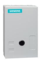
Electrically held lighting contactor, Contactor amp rating 30A, 0 N.C. / 4 N.O. Poles, 220VAC 50HZ/240VAC 60HZ coil, Non-combination type, (no disconnect device), Enclosure NEMA type 1, Indoor general purpose use
