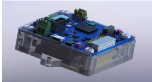
Figure 30. Core system board fastened with bolts
