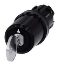
Key-operated switch BKS, 22 mm, round, plastic, special lock, with 2 keys, 3 switch positions I-O<II, latching on the left, momentary contact type on the right, actuating angle 2x45°, 10:30h/12h/13:30h, key removal O+I, Note: BKS locking systems E1 - E25 supplied without key
