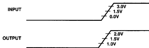
Figure 35. Voltage Reference Levels for AC Measurements (Except Output Enable/Disable)
