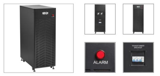
30kVA/kW transformer provides 480V (Delta) to 208V (Wye) step-down and isolation protection to a 3-phase UPS and its load.
