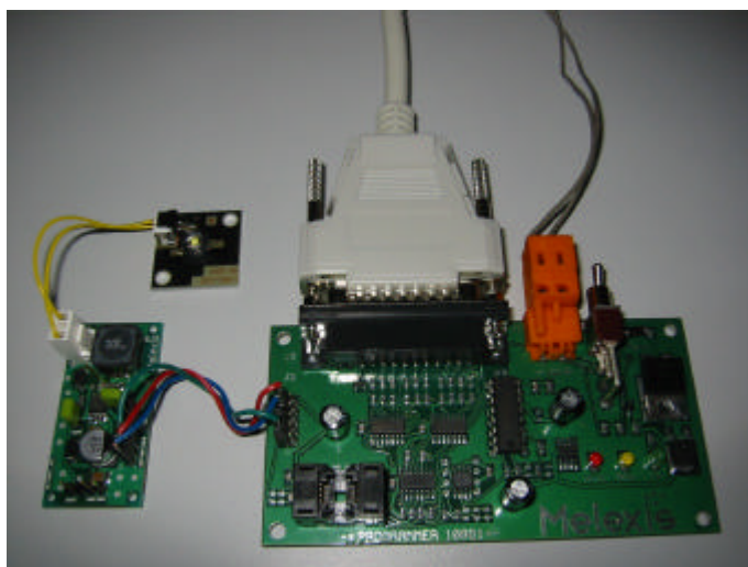
Figure 5: FL10801 connected to Melexis evaluation board EVB10801
