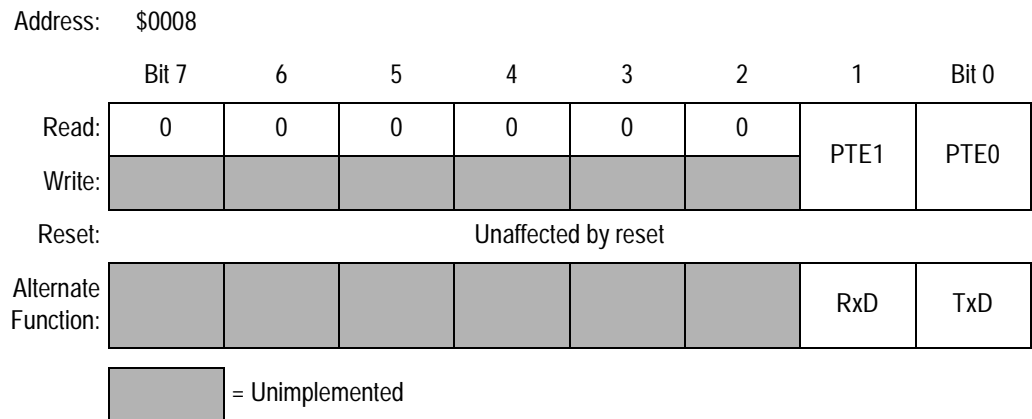
Figure 16-17. Port E Data Register (PTE)
