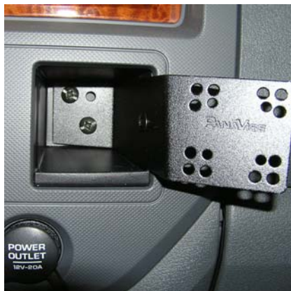
InDash Installed in Ram Pickup, Showing Screws and Location.
