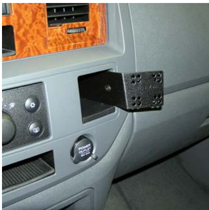
InDash Installed in Ram Pickup, Showing Screws and Location.
