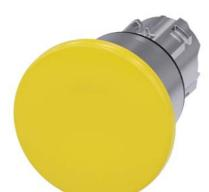
Mushroom pushbutton, 22 mm, round, metal, shiny, yellow, 40 mm, latching, pull-to-unlatch mechanism, with laser labeling, upper case
