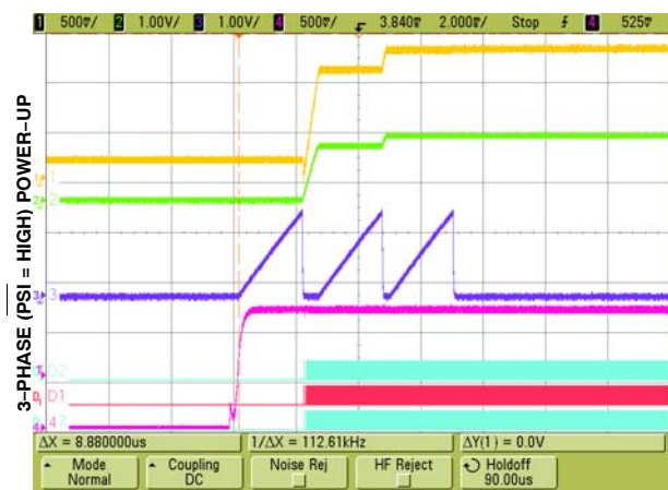
Figure 6. Typical Startup Waveform 1-Vo, 2-SS, 3-DELAY, 4-EN, D0-D3-PWM1~3
