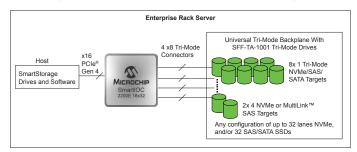
The Unified Smart Storage Solution means ease-of-management: manage mixed NVMe and SAS topologies with a single pane-of-glass.
