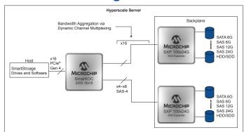
SmartIOC provides a new tier of storage fan-out with Dynamic Channel Multiplexed SAS-4 links to provide near 100% efficiency to targets such as SAS3 and SATA.
