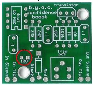
Step 6: Add the aluminum electrolytic capacitor. Your kit may come with a value between 1uf and 220uf. Aluminum electrolytic capcitors are polarized. The longer lead goes in the square solder pad.
