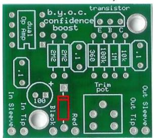
Step 2. Add the diode. The end with the stripe on it is called the cathode. This end goes into the square solder pade and stripe on the diode and stripe on the layout should match up. The other end of the diode is called the anode.
