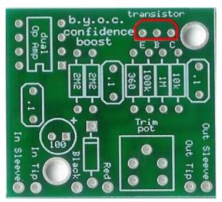
Step 5: Add the transistor. Match the curved side of the transistor up with the curve side of the layout. A TO-92 package transistor such as the 2N5088 will have 3 leads - the emmiter, base, and collector. They are marked on the PCB with E, B, and C.
