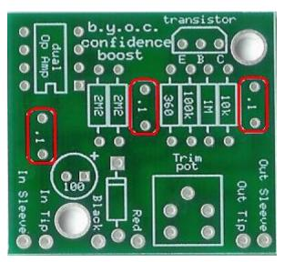
Step 7: Add the film capacitors. These are not polarized and can go in either direction.
