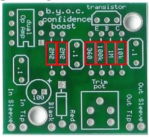
Step 1: Add the resistors. You want to add the components with the lowest profile first so that when you flip the PCB over to solder, the components don't fall out. Resistors are not polarized(polarized means it has a positive and negative end) so you can insert them into the board either way.
