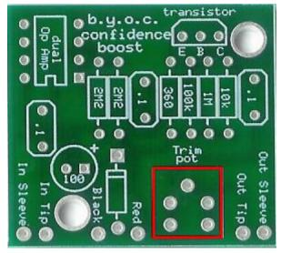
Step 4: Add the trimpot. The trimpot will have 3 leads. The PCB has eyelets for 5 leads. This is so that the PCB can accept a variety of pinout styles. There will only be one what the trimpot can fit into the PCB.
