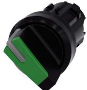
Selector switch, illuminable, 22 mm, round, plastic, green, selector switch, short, 2 switch positions O<I, momentary contact type, Actuating angle 45°, 10:30h/12h, with laser labeling, upper case and lower case, always upper case at the beginning of the word
