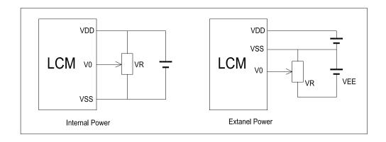
$V_{DD{\scriptscriptstyle \sim}} V_0 \hbox{: LCD Driving voltage}$
