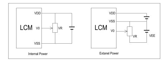
V<sub>DD∼</sub>V₀: LCD Driving voltage
