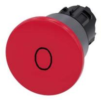
Mushroom pushbutton, 22 mm, round, plastic with metal front ring, red, inscription: O, 40 mm, latching, pull-to-unlatch mechanism, Z=50-unit packaging
