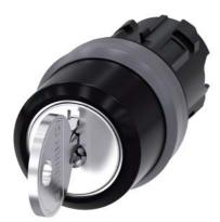
RONIS key-operated switch, 22 mm, round, plastic with metal front ring, lock number 455, with 2 keys, 3 switch positions I-O-II, latching, actuating angle 2x45°, 10:30h/12h/13:30h, Key removal I+O+II, Z=50-unit packaging
