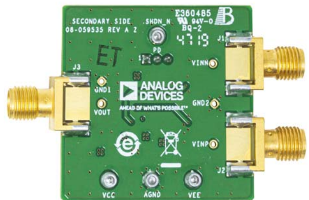
Figure 2. EVAL-LTC6228IS8, Secondary Side
