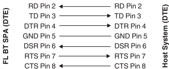
Figure 8 Assignment of 1:1 cables
