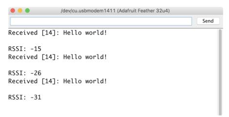
To receive a message simply call the **receive** function. This function will wait for half a second for any packet to be received. If a packet is found it will be returned as a byte string (remember packets are at most 60 bytes long), or if no packet was found a result of **None** is returned.
