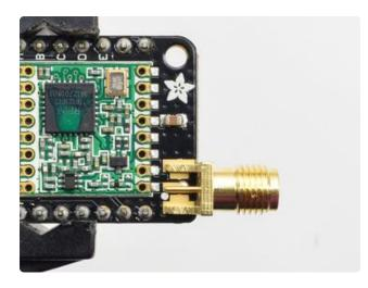
You'll need an SMA (or, if you need RP-SMA for some reason) Edge-Mount connector with 1.6mm spacing
