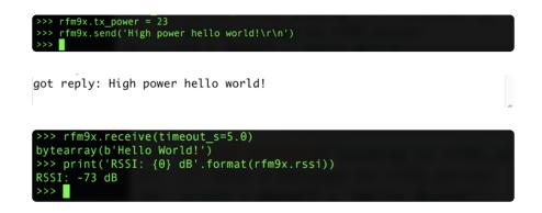
That's all there is to the basic RFM9x radio usage! Remember the CircuitPython module is designed for sending and receiving small up to 252 byte control messages and not large or high bandwidth amounts of data.
