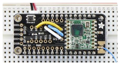
Because each Feather uses a different processor, there is some light wiring that needs to be done to configure the radio pins. In particular, an interrupt-capable pin is required for IRQ but there is no one irq pin that is the same on all the Feathers!
