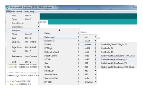
Before uploading, check for the #define FREQUENCY RF69\_915MHZ line and comment that out (and uncomment the line above) to match the frequency of the hardware you're using
