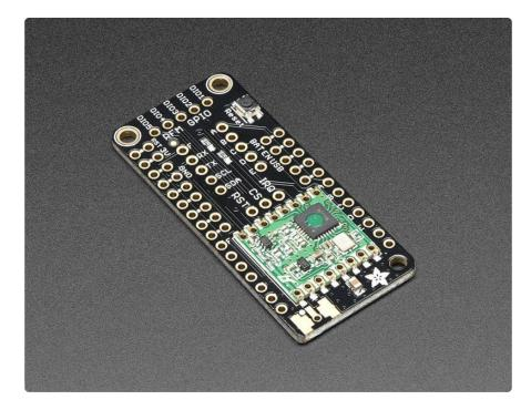
These radio modules come in four variants (two modulation types and two frequencies) The RFM69's are easiest to work with, and are well known and
