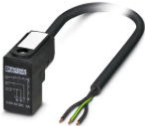
Sensor/Actuator cable, 3-position, PVC, Black RAL 9005, Free cable end, on C valve plug (8 mm), Cable length: 5 m
