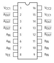
Pin assignment is for Dual-in-Line Package.
