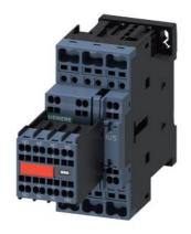
Power contactor, AC-3 32 A, 15 kW / 400 V 2 NO + 2 NC, 230 V AC 50/60 Hz, 3-pole Size S0, Spring type terminal Captive auxiliary switch
