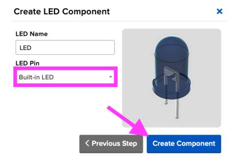
Behind the scenes, Adafruit IO sends send a command to your board running WipperSnapper telling it to configure the GPIO pin as a digital output. Your board's interface shows the new LED component.
