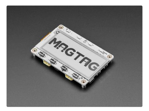
The Adafruit MagTag combines the new ESP32-S2 wireless module and a 2.9" grayscale E-Ink display to make a low-power IoT display that can show data on its screen even when power is removed! The ESP32-S2 is great because it builds on the years of code and support for the ESP32 and also adds native USB support so you can use this board with Arduino or CircuitPython!
