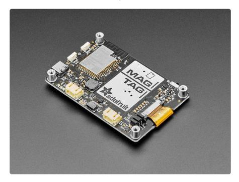
We designed this board to be low-power friendly - with a spot for a 350 or 420 mAh battery and built in battery charging over USB C. During deep sleep, with the
