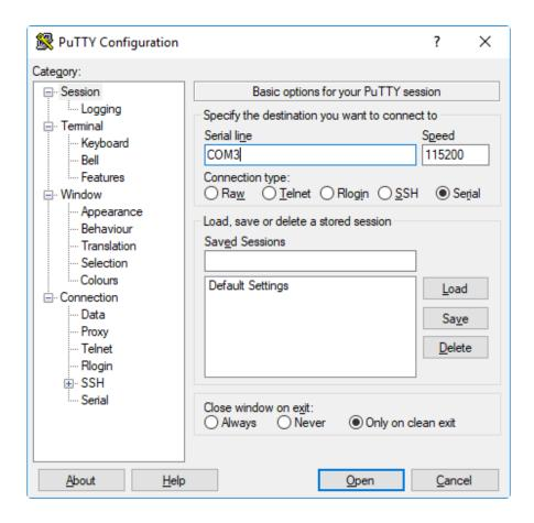
Once your settings are entered, you're ready to connect to the serial console. Click "Open" at the bottom of the window. A new window will open.
