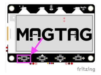
Button A is located towards the bottom left corner of the board. It is marked with both a left arrow and D15 on the silk.
