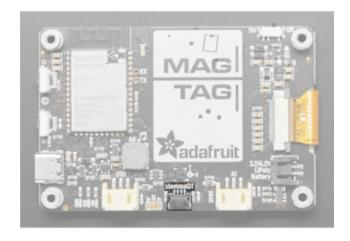
STEMMA QT () - This JST SH 4-pin connector breaks out I2C (SCL, SDA, 3.3V, GND). It allows you to connect to various breakouts and sensors with STEMMA QT connectors () or to other things using assorted associated accessories ().
