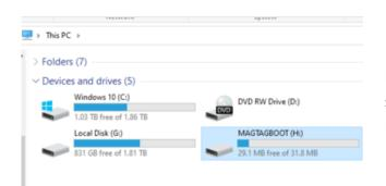
If the UF2 bootloader is installed, you will see a new disk drive appear called MAGTAGBOOT
