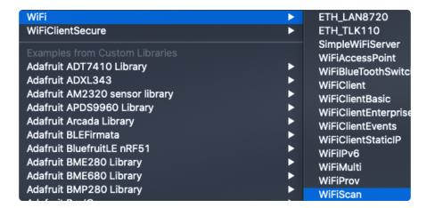
And upload this example to your board. The ESP32 should scan and find WiFi networks around you.
