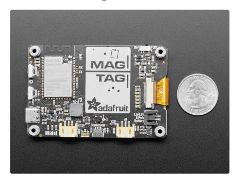
And of course, the Mag in MagTag stands for magnetic. We have four M3 standoffs that will work perfectly with these mini magnet feet. () (Originally they're designed for RGB Matrices but they'll do an excellent job here as well). Screw on the feet and you can attach this display to a metallic shelf, fridge, or bench.
