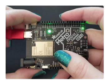
Before we upload a sketch, place your ESP32-S2/S3 board into ROM bootloader mode ().
