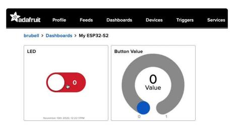
You should also see the ESP32-S2/S3's LED turning on and off when the LED is toggled:
