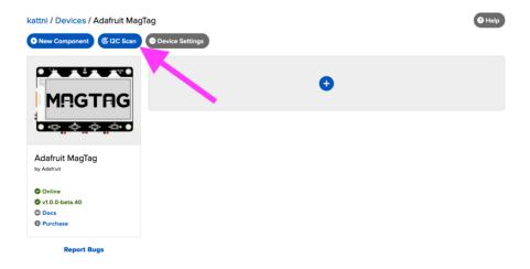
You should see a new pop-up showing a list of the I2C addresses detected by an I2C scan. If wired correctly, the AHT20's default I2C address of 0x38 appear in the I2C scan list.
