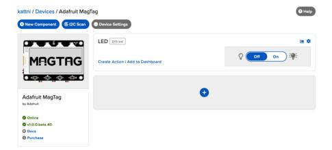
On the device interface, toggle the LED component by clicking the toggle switch. This should turn your board's built-in LED on or off.
