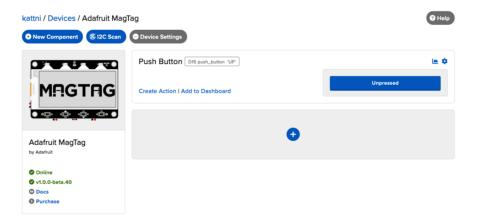
Press the button to change the value of the push button component on Adafruit IO.
