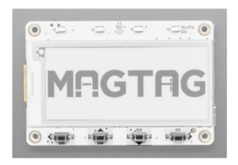
On the front of the board, along the bottom, there are four user-controllable buttons labeled both with pin names and a different arrow for each button. The buttons are on D11, D12, D14 and D15. Can be used to wake up the ESP32-S2 from deep-sleep, or select different modes.
