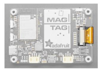
Front and center is a 2.9" grayscale elnk display with 296x128 pixels. Each pixel can be white, light gray, dark gray or black. For use with general Arduino libraries, you can try GxEPD2\_290\_T5 - the Arduino library Adafruit uses is
