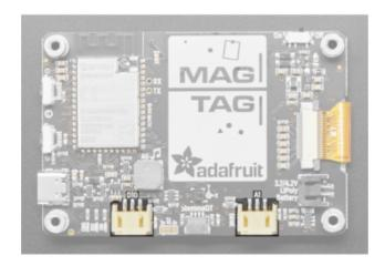
On the bottom are two connectors labeled D10 and A1. These are STEMMA 3 pin JST digital or analog connectors for attaching NeoPixels (), speakers (), servos () or relays (). These pins can be analog inputs or digital I/O.
