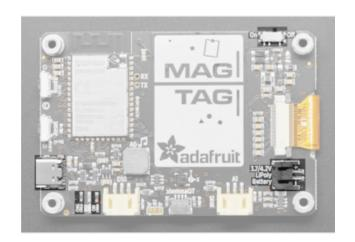
There are two ways to power the MagTag board: the USB type C connector or a 3.7/4.2V Lipoly battery.
