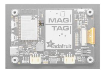
The hardware UART debug port has two broken out pins. You can connect these to a USB console cable in order to read the debug output from the ESP32 IDF (). This is useful if you are writing software and need to see the low level debug output.
