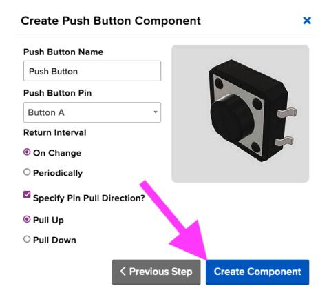
Adafruit IO should send a command to your board (running WipperSnapper), telling it to configure the GPIO pin you selected to behave as a digital input pin and to enable it to pull up the internal resistor. Your board's interface should also show the new push-button component.
