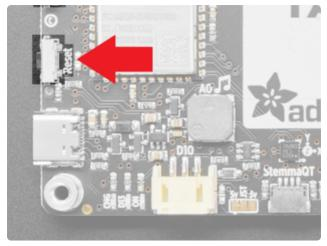
Launch UF2 by double-clicking the Reset button (the one next to the USB C port). You may have to try a few times to get the timing right.
