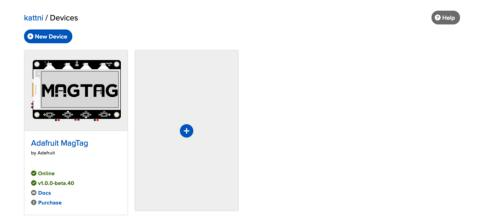
Once verified that the device is online, click the device tile to navigate to the device's interface page.
