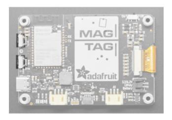
Reset button - The reset button in the top left corner is used to reset the board. Boot0 button - This is connected to BOOT0 and can be used to put the board into ROM bootloader mode. To enter ROM bootloader mode, hold down the BOOT0 button while clicking reset button mentioned above. When in the ROM bootloader, you can upload code and query the chip using esptool.
