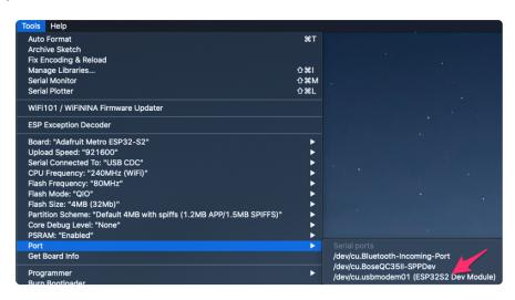
Do not select any other port than the one that is called "ESP32S2 Dev Module" or "ESP32S3 Dev Module"
