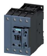
Power contactor, AC-3 50 A, 22 kW / 400 V 2 NO + 2 NC 24 V AC, 50/60 Hz 4-pole size S2 screw terminals 1 NO + 1 NC integrated
