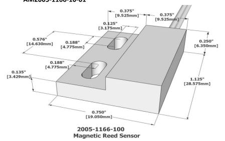
All measurements are in Inches [millimeters]
