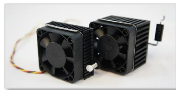
There are variations in fin density and length between convection types even when it is a very similar construction.
