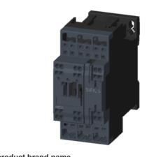
power contactor, AC-3 25 A, 11 kW / 400 V 1 NO + 1 NC, 110 V AC, 50 / 60 Hz, 3-pole, Size S0, Spring-type terminal
