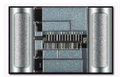
This Precision Laser Trimmed Capacitor (PLTC) provides an excellent solution for applications requiring precision tunable capacitance in a surface mount LGA package. It has been designed with stable SiON dielectric in combination with finely tunable capacitor ladder structures.
