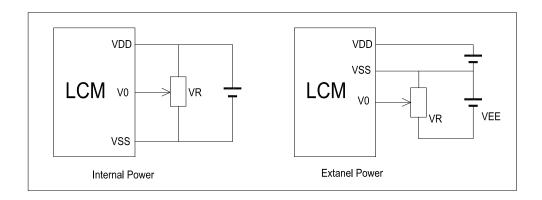
$V_{DD{\scriptscriptstyle \sim}} V_0 \hbox{: LCD Driving voltage}$
