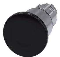
Mushroom pushbutton, 22 mm, round, metal, shiny, black, 40 mm, 3 switch positions, latches after pushing in, unlatches by pull-to-unlatch mechanism to center position, after pulling out the button Retraction to center position, with laser labeling, inscription or symbol Customer-specific selection with SIRIUS ACT configurator (CIN)
