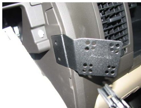
InDash Installation Location
