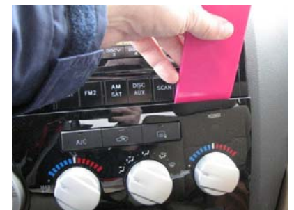
AC Bezel released w/ Dash Tool
