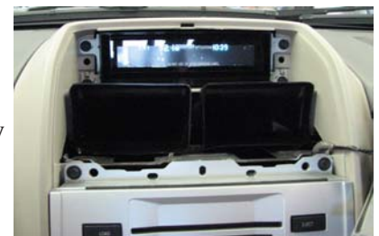
Air Vent Assembly Removed
