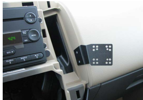
InDash Installed, Mounting Location - Edge
