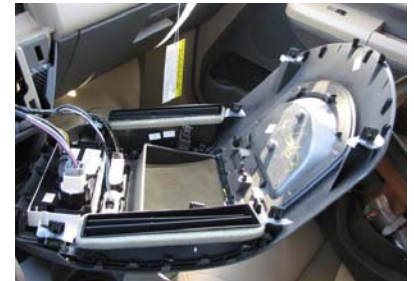
Radio Climate Control, Air Vent, Bezel Removed
