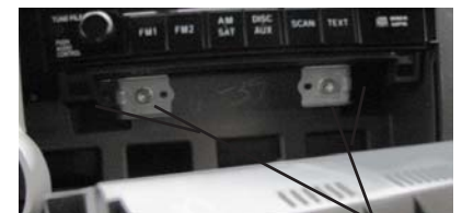
(4) Radio bolts Location
