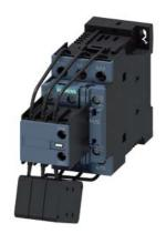
Capacitor contactor, AC-6b 16.7 kVAr, / 400 V 1 NO + 2 NC, 24 V DC 3-pole, Size S0 screw terminal
