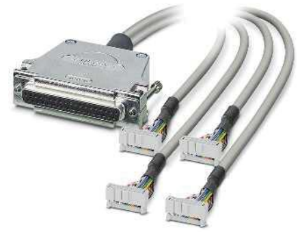
Splitting cable, D-SUB socket strip to IDC/FLK socket strip, number of positions 37 to 4 x 14
