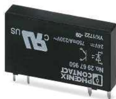
Solid-state relay, AC output max. 750 mA
