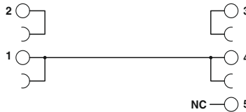
Connection scheme PLC-VT
