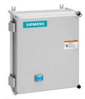
Non-reversing motor starter, Size 1, Three phase full voltage, Solid-state overload relay, OLR amp range 5.5-22A, Non-combination type, Enclosure type 4X fiberglass, Water/dust tight noncorrosive, Standard width enclosure
