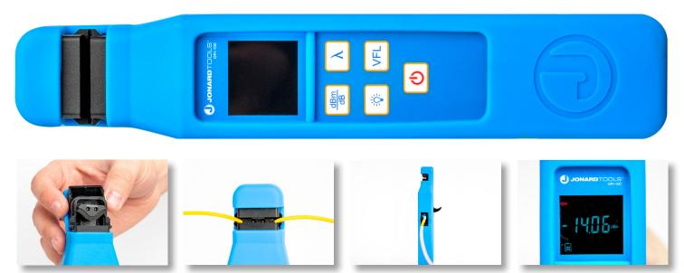
Designed to quickly identify the direction of light being transmitted in the fiber and display the relative core power without damaging the fiber. This fiber identifier is the perfect tool for identifying fiber in network systems without disrupting the network and includes a built-in VFL and Power Meter for convenience. This fiber identifier also features the following:
