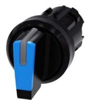
Selector switch, illuminable, 22 mm, round, plastic, blue, selector switch, short, 3 switch positions I>O<II, momentary contact type, actuating angle 2x45°, 10:30h/12h/13:30h, with laser labeling, upper case and lower case, always upper case at beginning of line
