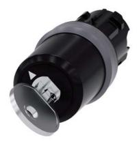
key-operated switch Siemens, 22 mm, round, plastic with metal front ring, lock number SSG10, with 2 keys, 2 switch positions O-I, latching, actuating angle 90°, 10:30h/13:30h, key removal O+I, Z=50-unit packaging
