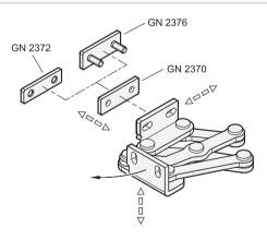
Multiple-joint hinges can be adjusted in three planes during installation. For example, this allows compensation for tolerances or establishing of required compressive forces for seals.
